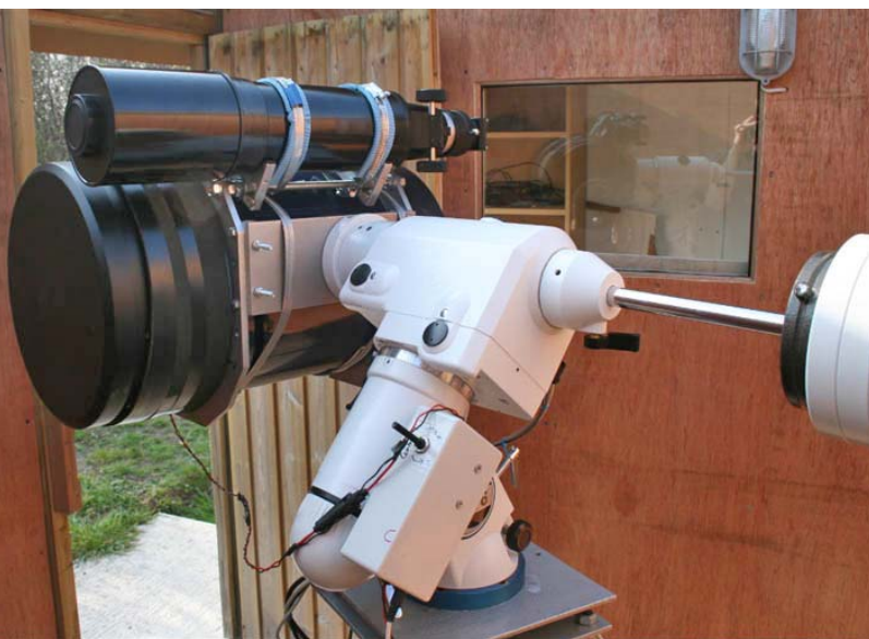
Figure 1. The telescope used to collect the data presented in this paper. 0.25m SCT with 0.1m refractor guidescope, mounted on an EQ6 in a simple roll-off-roof observatory.
